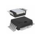
VND830LSP **Description:** IC DRIVR DUAL 36V 18A POWERSO-10 Manufacturers: STMicroelectronics In Stock: New original, 5700 pcs Stock Available.
