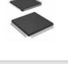
C8051F022-GQR Description: IC MCU 8BIT 64KB FLASH 100TQFP Manufacturers: Energy Micro (Silicon Labs) In Stock: New original, 400 pcs Stock Available.
