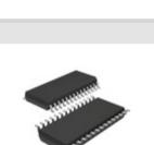
ADM241LJRS **Description:** IC TXRX RS-232 4:5 5V LP 28SSOP Manufacturers: ADI (Analog Devices, Inc.) In Stock: New original, 4800 pcs Stock Available.
