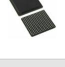
PI7C8150DNDE Description: IC PCI-PCI BRIDGE ASYNC 256BGA
