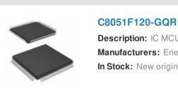
Description: IC MCU 8BIT 128KB FLASH 100TQFP Manufacturers: Energy Micro (Silicon Labs) In Stock: New original, 2000 pcs Stock Available. RFQ
