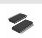
FIN1532MTC Description: IC RCVR QUAD 5V HS LVDS 16TSSOP Manufacturers: AMI Semiconductor / ON Semiconductor
