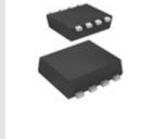
**AON3613** Description: MOSFET N/P-CH 30V 4.5A 8DFN Manufacturers: Alpha and Omega Semiconductor, Inc.
