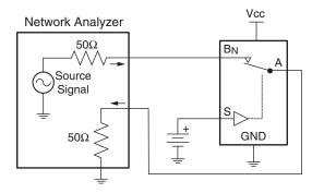
Figure 6. ON/Off Capacitance Measurement
