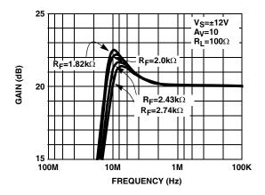
FIGURE 5. DRIVER DIFFERENTIAL FREQUENCY RESPONSE vs R<sub>F</sub> (TERMINATE MODE)
