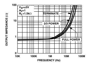
FIGURE 18. OUTPUT IMPEDANCE vs FREQUENCY
