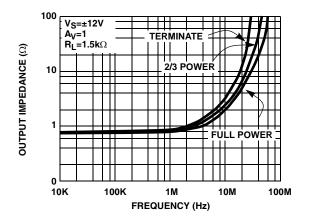
FIGURE 17. OUTPUT IMPEDANCE vs FREQUENCY
