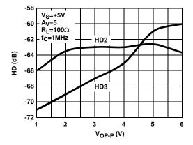
FIGURE 28. DIFFERENTIAL HARMONIC DISTORTION vs OUTPUT AMPLITUDE (2/3 POWER)
