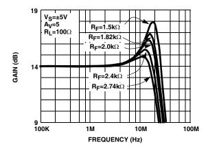
FIGURE 10. DRIVER DIFFERENTIAL FREQUENCY RESPONSE vs R<sub>F</sub> (2/3 POWER MODE)
