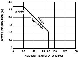
FIGURE 38. POWER DISSIPATION vs AMBIENT TEMPERATURE
