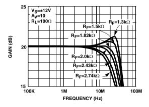
FIGURE 1. DRIVER DIFFERENTIAL FREQUENCY RESPONSE vs R<sub>F</sub> (FULL POWER MODE)
