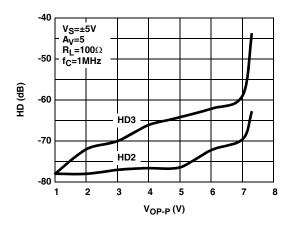
FIGURE 22. DIFFERENTIAL HARMONIC DISTORTION vs **OUTPUT AMPLITUDE**
