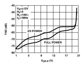
FIGURE 23. DIFFERENTIAL TOTAL HARMONIC DISTORTION vs OUTPUT AMPLITUDE
