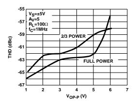
FIGURE 30. DIFFERENTIAL TOTAL HARMONIC DISTORTION vs OUTPUT AMPLITUDE
