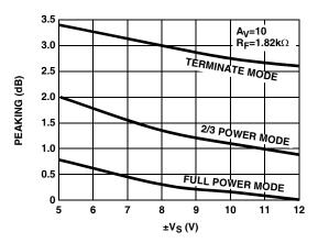
FIGURE 32. DIFFERENTIAL PEAKING vs SUPPLY VOLTAGE
