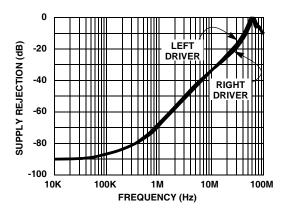
FIGURE 15. POSITIVE SUPPLY REJECTION vs FREQUENCY
