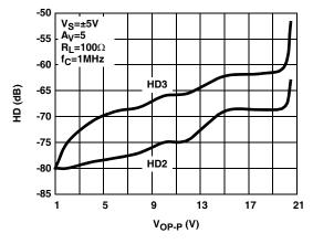
FIGURE 21. DIFFERENTIAL HARMONIC DISTORTION vs **OUTPUT AMPLITUDE (2/3 POWER)**
