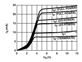
FIGURE 14. SUPPLY CURRENT vs SUPPLY VOLTAGE
