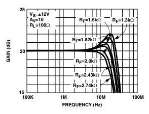
FIGURE 3. DRIVER DIFFERENTIAL FREQUENCY RESPONSE vs  $R_F$  (2/3 POWER MODE)
