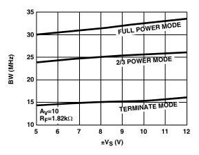
FIGURE 31. DIFFERENTIAL BANDWIDTH vs SUPPLY VOLTAGE
