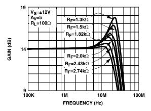
FIGURE 9. DRIVER DIFFERENTIAL FREQUENCY RESPONSE vs R<sub>F</sub> (2/3 POWER MODE)
