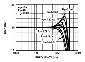
FIGURE 2. DRIVER DIFFERENTIAL FREQUENCY RESPONSE vs R<sub>F</sub> (FULL POWER MODE)
