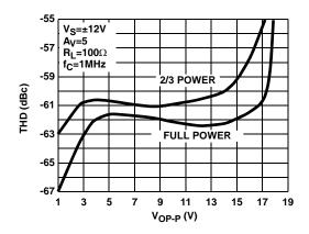
FIGURE 29. DIFFERENTIAL TOTAL HARMONIC DISTORTION vs OUTPUT AMPLITUDE
