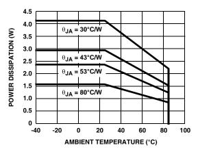
FIGURE 37. POWER DISSIPATION vs AMBIENT TEMPERATURE for VARIOUS MOUNTED  $\theta_{\mbox{\scriptsize JAS}}$
