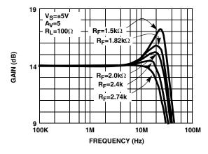
FIGURE 8. DRIVER DIFFERENTIAL FREQUENCY RESPONSE vs R<sub>F</sub> (FULL POWER MODE)
