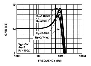
FIGURE 12. DRIVER DIFFERENTIAL FREQUENCY RESPONSE vs R<sub>F</sub> (TERMINATE MODE)
