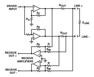
FIGURE 39. TYPICAL LINE INTERFACE CONNECTION
