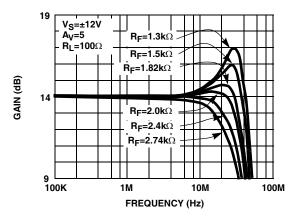
FIGURE 7. DRIVER DIFFERENTIAL FREQUENCY RESPONSE vs R<sub>F</sub> (FULL POWER MODE)
