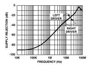
FIGURE 16. NEGATIVE SUPPLY REJECTION vs FREQUENCY
