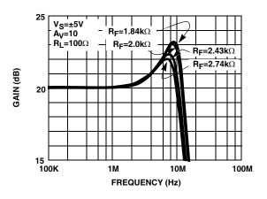
FIGURE 6. DRIVER DIFFERENTIAL FREQUENCY RESPONSE vs R<sub>F</sub> (TERMINATE MODE)
