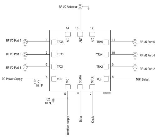
Figure 6. SKY13526-485LF Evaluation Board Schematic
