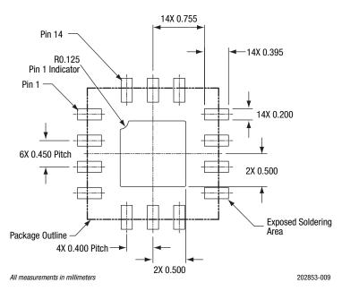
Figure 9. SKY13526-485LF PCB Layout Footprint (Top View)
