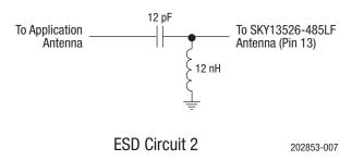
Figure 7. SKY13526-485LF Recommended ESD Protection Circuits
