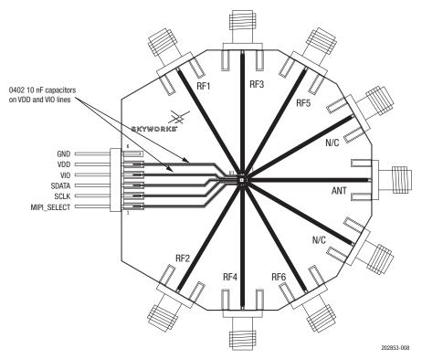
Figure 8. SKY13526-485LF Evaluation Board Assembly Diagram
