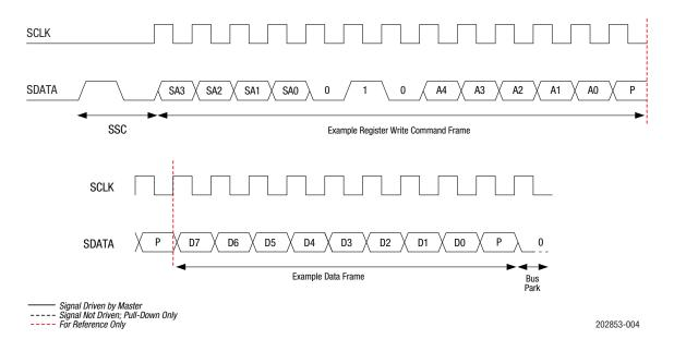
**Figure 4. Register Write Command Timing Diagram**
