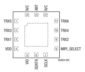
Figure 2. SKY13526-485LF Pinout (Top View)
