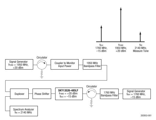
**Figure 3. Third Order Intermodulation Test Setup**
