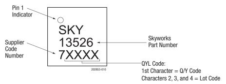
Figure 10. Typical Part Marking (Top View)
