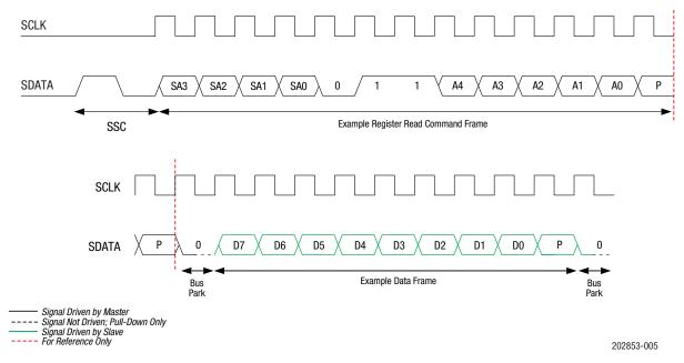
**Figure 5. Register Read Command Timing Diagram**
