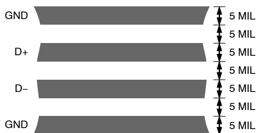
Figure 23. Typical Arrangement of Signal Tracks
