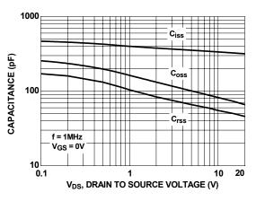
Figure 8. Capacitance Characteristics
