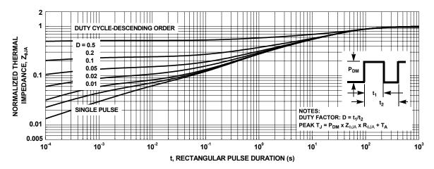
Figure 13. Transient Thermal Response Curve
