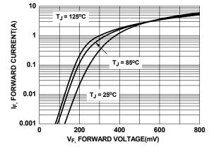
Figure 11. Schottky Diode Forward Current
