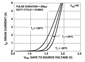
Figure 5. Transfer Characteristics
