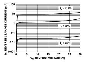
Figure 12. Schottky Diode Reverse Current
