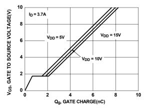
Figure 7. Gate Charge Characteristics
