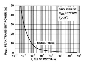
Figure 10. Single Pulse Maximum Power Dissipation
