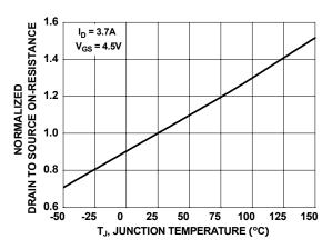
Figure 3. Normalized On-Resistance vs Junction Temperature
