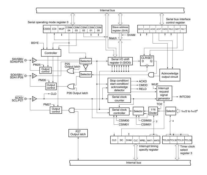
Figure 17-2. Block Diagram of Serial Interface Channel 0
