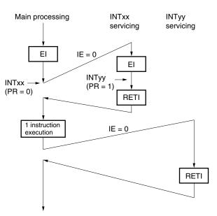
INTyy, which occurs while INTxx is being serviced is not acknowledged for multiple interrupt servicing because the priority of INTyy is lower than that of INTxx. INTyy is held pending and is acknowledged after one instruction of the main processing has been executed.
