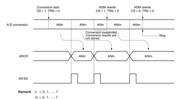
Figure 14-8. A/D Conversion by Software Start
