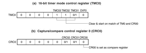
**Remark** 0/1: Setting 0 or 1 allows another function to be used simultaneously with the external event counter. See the description of the respective control registers for details.
