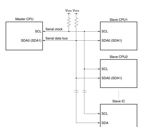
Figure 17-13. Example of Serial Bus Configuration Using I<sup>2</sup>C Bus
