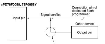
In the flash memory programming mode, the signal output by another device and the signal sent by the dedicated flash programmer conflict, therefore, isolate the signal of the other device.
