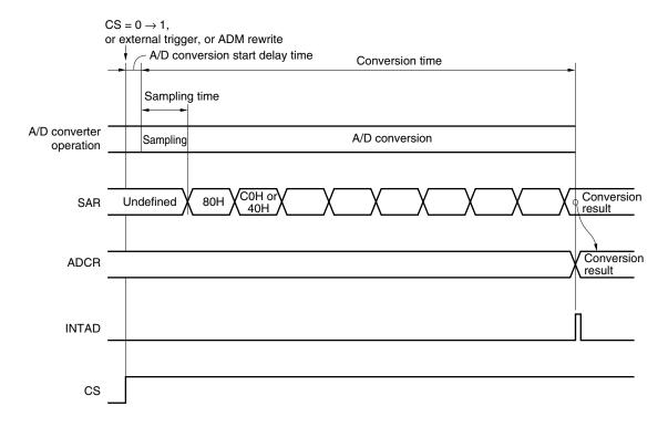
A/D conversion operations are performed continuously until bit 7 (CS) of the AD converter mode register (ADM) is reset to 0 by software.
