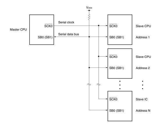
Caution When exchanging the master CPU/slave CPU, a pull-up resistor is necessary for the serial clock line ( $\overline{SCK0}$ ) as well because serial clock line ( $\overline{SCK0}$ ) input/output switching is carried out asynchronously between the master and slave CPUs.
