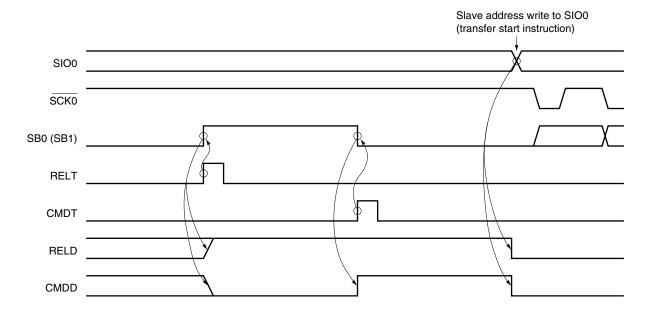
Figure 16-20. RELT, CMDT, RELD, and CMDD Operations (Master)
