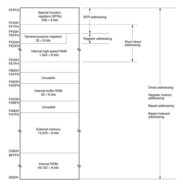
Figure 5-10. Data Memory Addressing (µPD780056, 780056(A), 780056Y, 780056Y(A))
