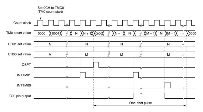
Caution The 16-bit timer register starts operation at the moment TMC01 to TMC03 are set to values other than 0, 0, 0 (operation stop mode).
