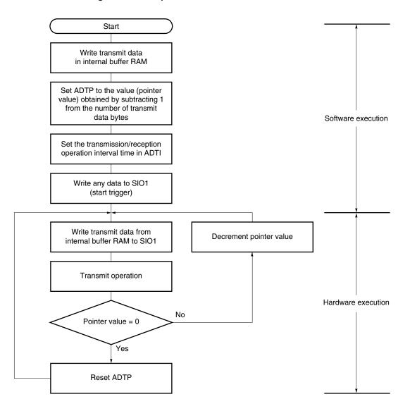
Figure 18-15. Repeat Transmission Mode Flowchart
