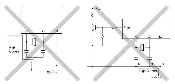
**Remark** When using the subsystem clock, replace X1 and X2 with XT1 and XT2, respectively. Also, insert resistors in series on the XT2 side.
