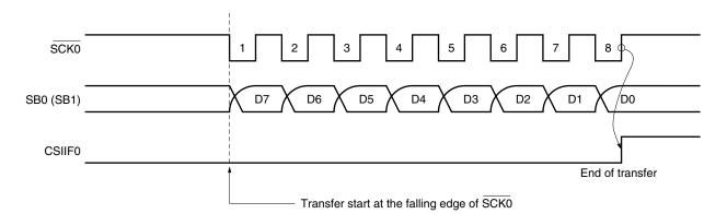
Figure 16-32. 2-Wire Serial I/O Mode Timing
