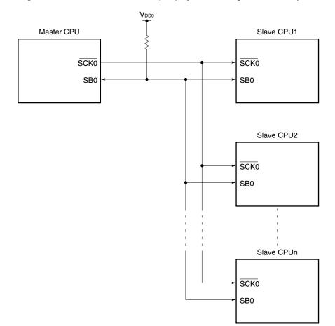
Figure 16-1. Serial Bus Interface (SBI) System Configuration Example
