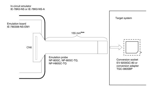
**Note** When NP-H80GC-TQ is used, the distance is 355 mm.
