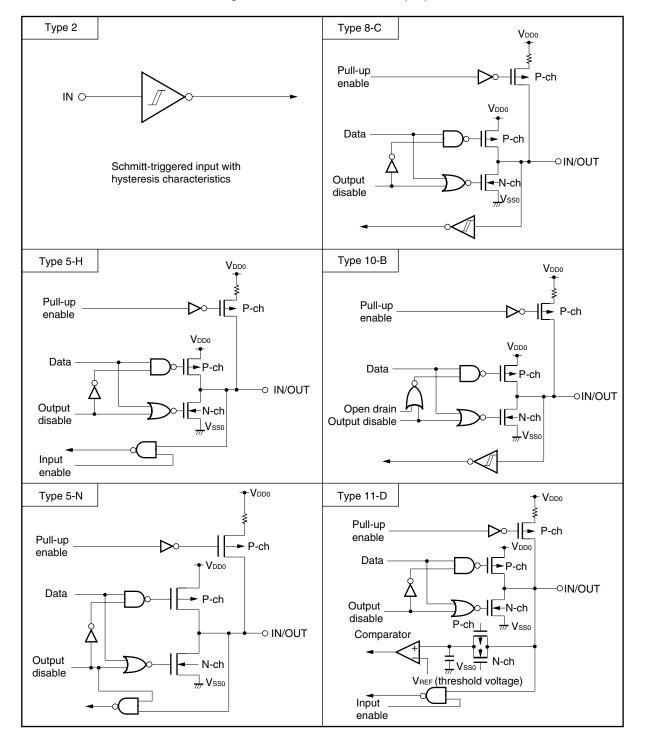
Figure 3-1. Pin I/O Circuit List (1/2)
