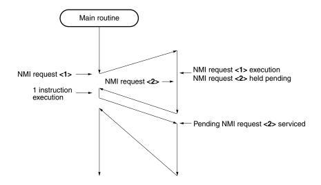
(b) If two non-maskable interrupt requests are generated during non-maskable interrupt servicing program execution
