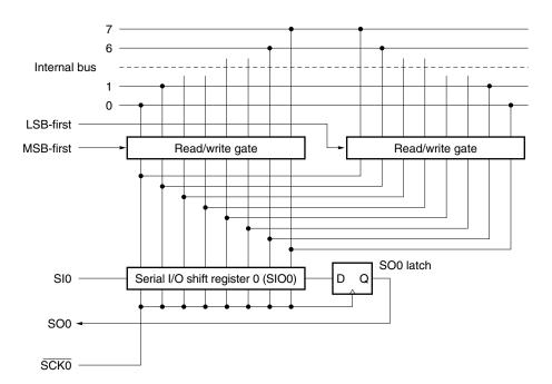
Figure 17-9. Circuit for Switching Transfer Bit Order
