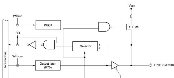
Figure 6-15. Block Diagram of P70
