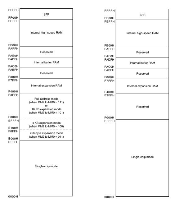
Caution When the internal ROM (flash memory) size is 60 KB, the area from F000H to F3FFH cannot be used. F000H to F3FFH can be used as external memory by setting the internal ROM (flash memory) size to 56 KB or less using the internal memory size switching register (IMS).
