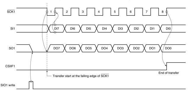
Figure 18-6. 3-Wire Serial I/O Mode Timing
