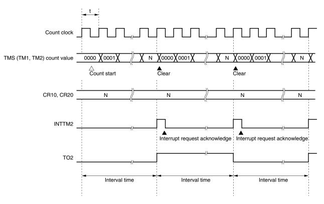
Figure 9-11. Interval Timer Operation Timing
