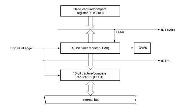
Figure 8-29. External Event Counter Configuration Diagram
