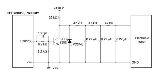
Figure 8-15. TV Tuner Application Circuit Example
