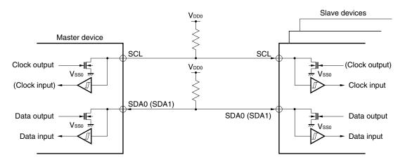
Caution To receive data, the N-ch open-drain output must made to go into a high-impedance state. Therefore, set bit 7 (BSYE) of the serial bus interface control register (SBIC) to 1 in advance, and write FFH to serial I/O shift register 0 (SIO0).
