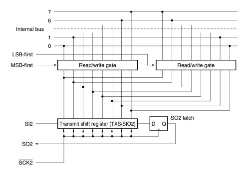
Figure 19-14. Circuit for Switching Transfer Bit Order
