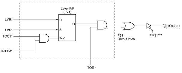
Figure 9-2. Block Diagram of 8-Bit Timer/Event Counter Output Controller 1
