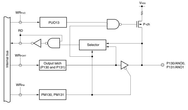
Figure 6-18. Block Diagram of P130 and P131
