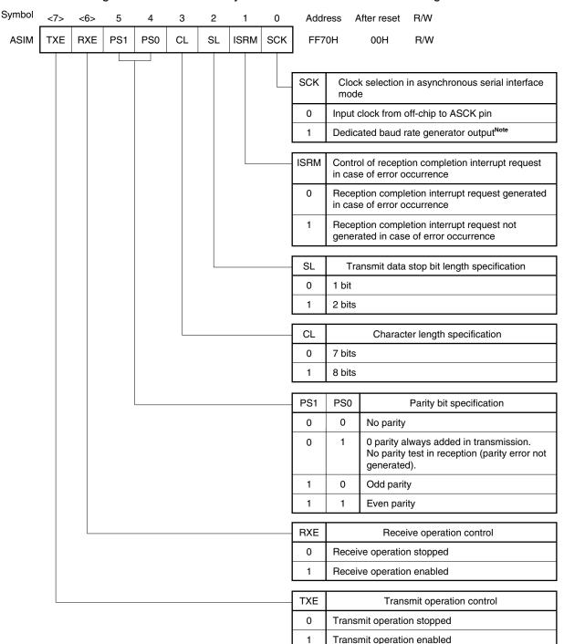
Figure 19-4. Format of Asynchronous Serial Interface Mode Register
