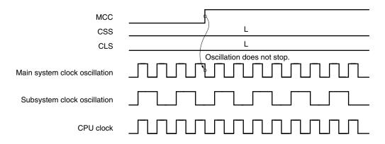
Figure 7-9. Main System Clock Stop Function (2/2)
