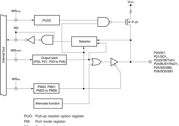
Figure 6-5. Block Diagram of P20, P21, and P23 to P26
