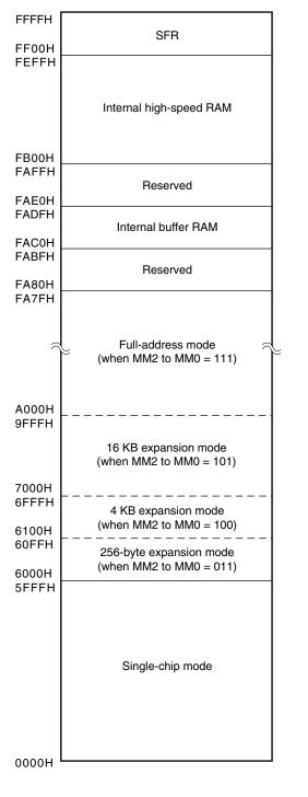
(b) Memory map of  $\mu$ PD780054 and 780054Y, and  $\mu$ PD780058, 780058B, 780058BY, 78F0058, and 78F0058Y with internal ROM (flash memory) set to 32 KB
