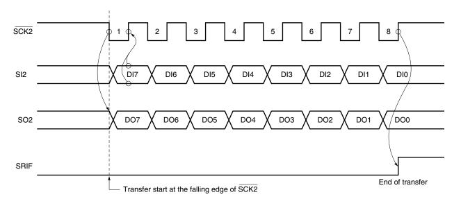
Figure 19-13. 3-Wire Serial I/O Mode Timing
