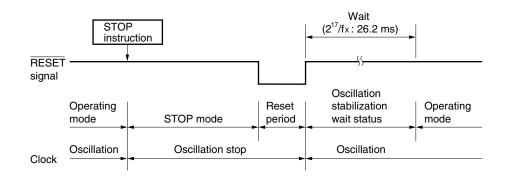
Figure 23-5. STOP Mode Release by RESET Input
