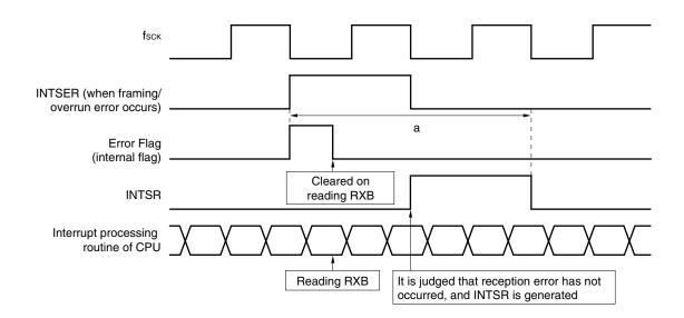
Remark ISRM: Bit 1 of the asynchronous serial interface mode register (ASIM)
