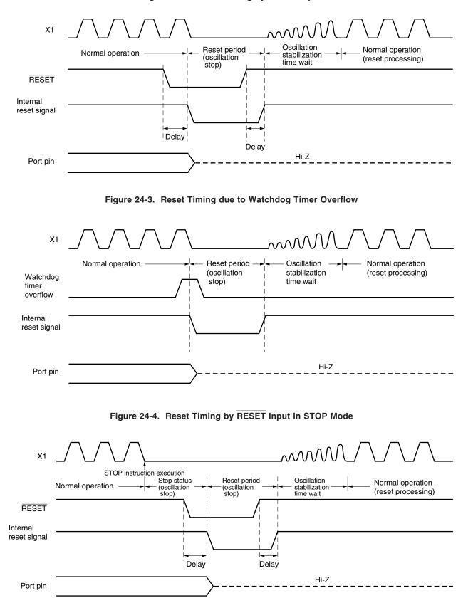
Figure 24-2. Reset Timing by RESET Input
