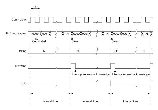
**Remark** Interval time =  $(N + 1) \times t : N = 0001H$  to FFFFH.
