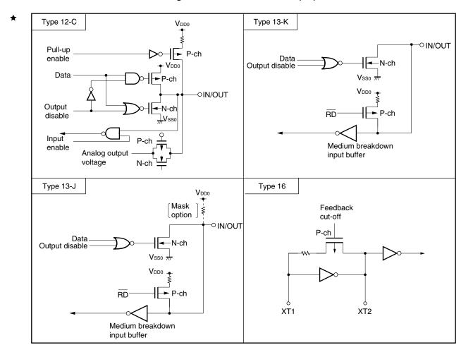
Figure 4-1. Pin I/O Circuit List (2/2)
