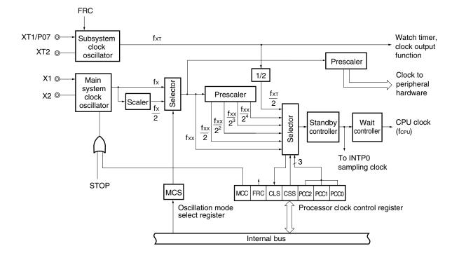
Figure 7-1. Clock Generator Block Diagram
