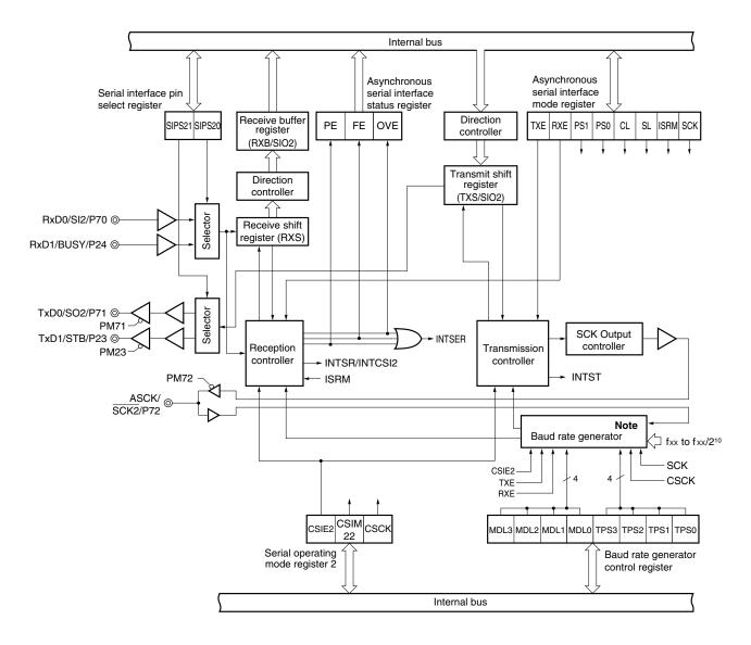
Figure 19-1. Block Diagram of Serial Interface Channel 2
