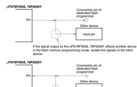
If the signal output by the dedicated flash programmer affects another device in the flash memory programming mode, isolate the signals of the other device.
