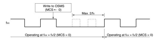
2. When writing 1 to MCS, VDD must be 2.7 V or higher before the write operation.
