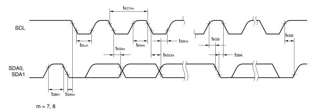
3-wire serial I/O mode with automatic transmit/receive function:
