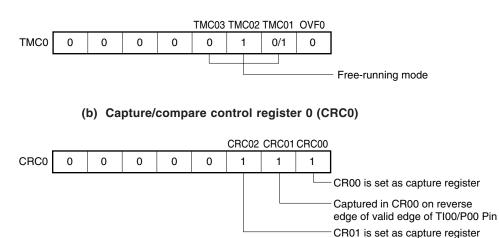
**Remark** 0/1: Setting 0 or 1 allows another function to be used simultaneously with pulse width measurement. See the description of the respective control registers for details.
