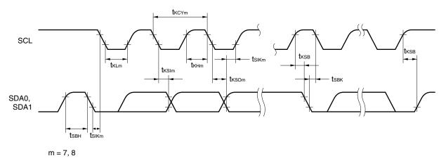
3-wire serial I/O mode with automatic transmit/receive function:
