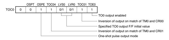
Remark 0/1: Setting 0 or 1 allows another function to be used simultaneously with one-shot pulse output. See the description of the respective control registers for details.
