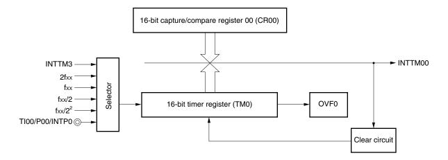
Figure 8-12. Interval Timer Operation Timings
