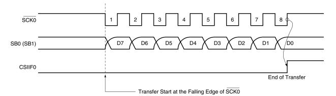
Figure 17-11. 2-Wire Serial I/O Mode Timing
