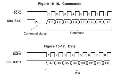
8-bit data following a command signal is defined as "command" data. 8-bit data without a command signal is defined as "data". Command and data operation procedures can be determined by the user according to their communication specifications.
