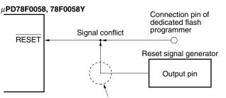
The signal output by the reset signal generator and the signal output from the dedicated flash programmer conflict in the flash memory programming mode, so isolate the signal of the reset signal generator.
