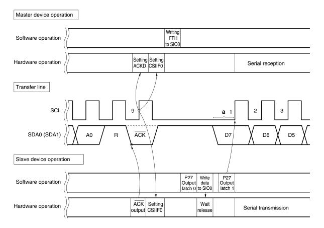
Figure 17-25. Slave Wait Release (Transmission)
