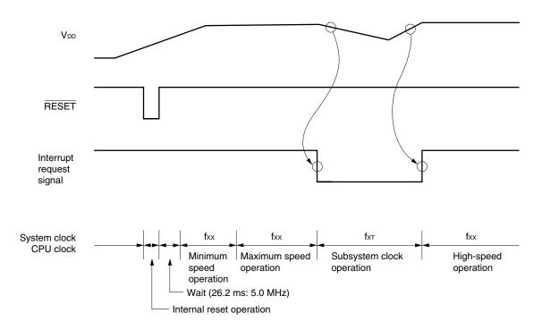
Figure 7-10. Switching Between System Clock and CPU Clock
