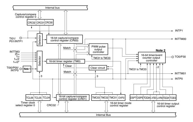
Figure 8-1. Block Diagram of 16-Bit Timer/Event Counter
