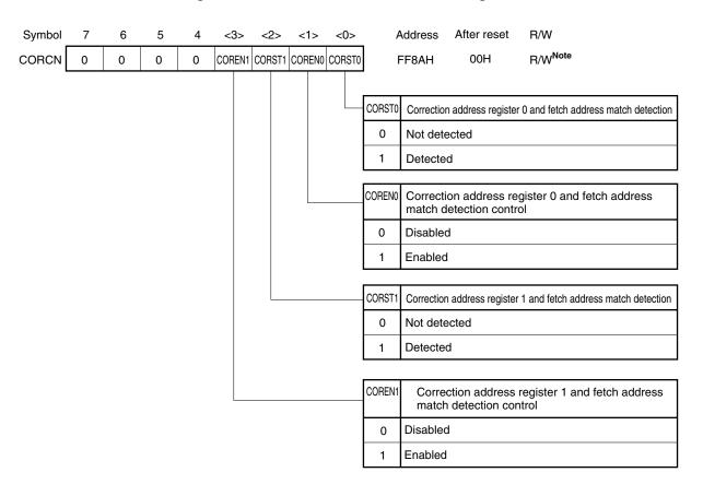
Figure 25-3. Format of Correction Control Register
