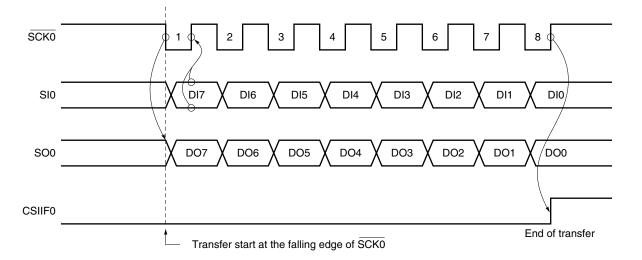
Figure 16-7. 3-Wire Serial I/O Mode Timing
