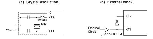
Caution When using a main system clock oscillator and a subsystem clock oscillator, carry out wiring
