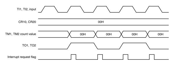
Figure 9-15. External Event Counter Operation Timing
