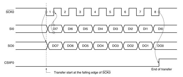
Figure 17-7. 3-Wire Serial I/O Mode Timing
