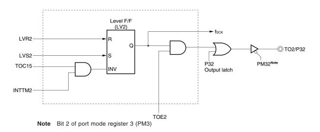
$\ensuremath{\textit{Remarks}}$  1. The section in the broken lines is the output controller.
