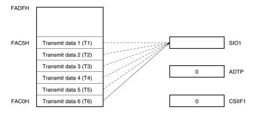
(b) Upon completion of transmission of 6 bytes
