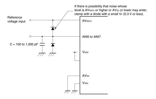
Figure 14-12. Analog Input Pin Handling
