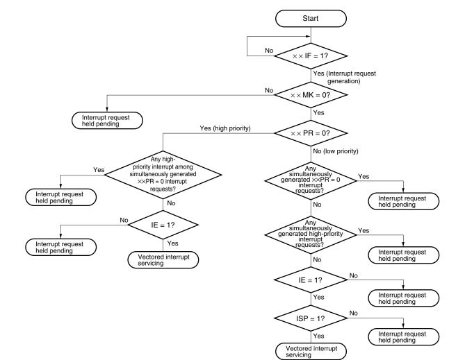
Figure 21-13. Interrupt Request Acknowledgment Processing Algorithm
