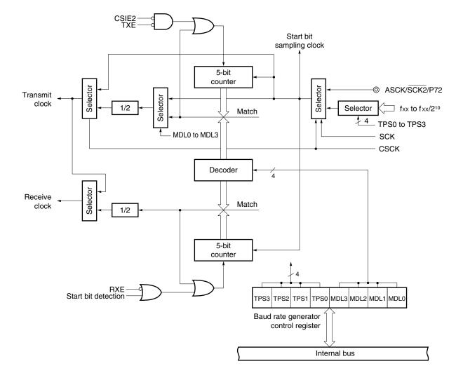
Figure 19-2. Baud Rate Generator Block Diagram
