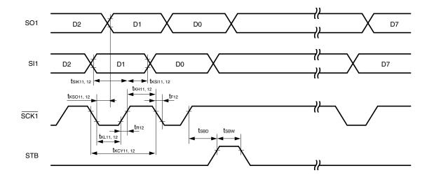
3-wire serial I/O mode with automatic transmit/receive function (busy processing):
