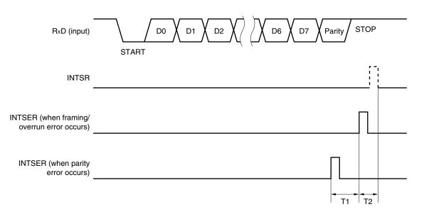
T1: Time of one data of baud rate selected by baud rate generator control register (BRGC) (1/baud rate)
