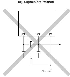
Figure 7-8. Examples of Resonator with Bad Connection (2/2)
