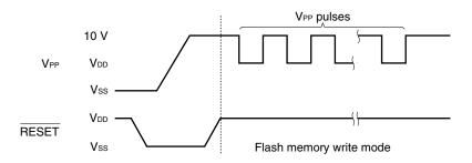
Figure 26-4. Communication Mode Selection Format
