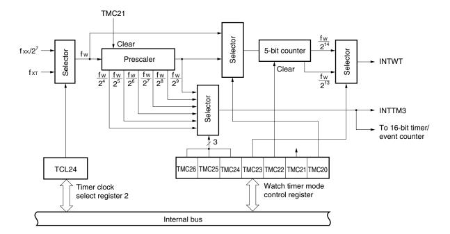
Figure 10-1. Watch Timer Block Diagram
