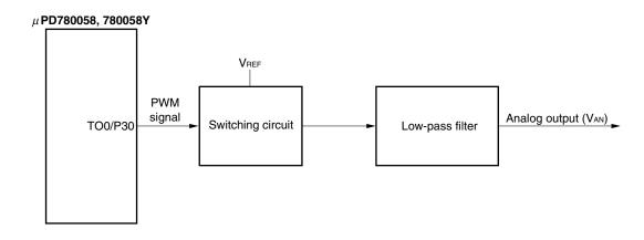
Figure 8-15 shows an example in which PWM output is converted to an analog voltage and used in a voltage synthesizer type TV tuner.
