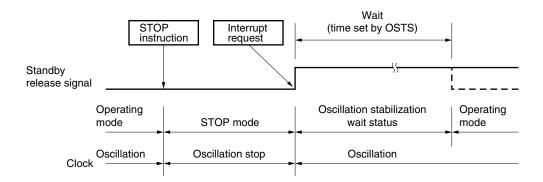
**Remark** The broken lines indicate the case when the interrupt request which has released the standby status is acknowledged.
