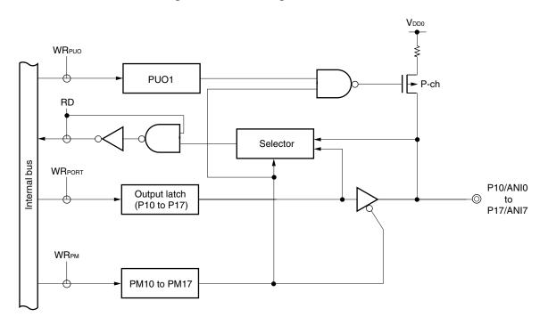
Figure 6-4. Block Diagram of P10 to P17
