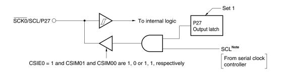
Note The level of the SCL signal is in accordance with the contents of the logic circuits shown in Figure 17-29.
