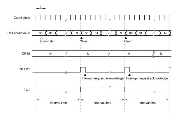
Figure 9-8. Interval Timer Operation Timing
