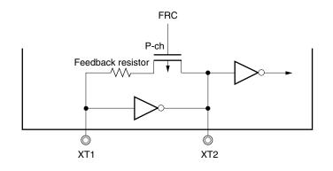
Figure 7-2. Subsystem Clock Feedback Resistor
