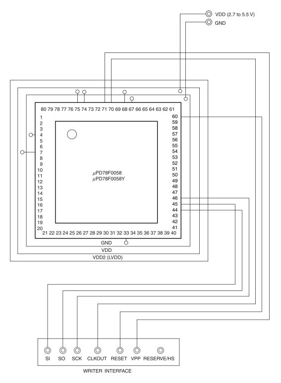
Figure 26-15. Wiring Example for Flash Writing Adapter in Pseudo 3-Wire Mode
