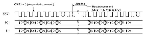
Figure 18-17. Automatic Transmission/Reception Suspension and Restart
