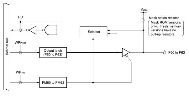
Figure 6-13. Block Diagram of P60 to P63
