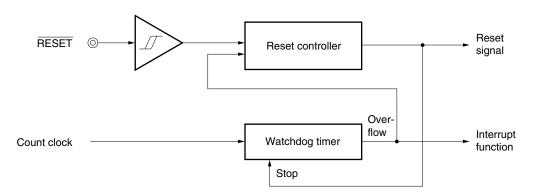
Figure 24-1. Reset Function Block Diagram
