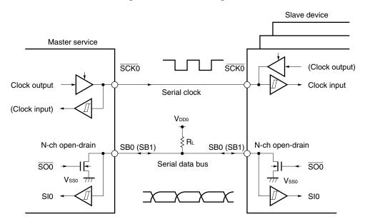
Figure 16-26. Pin Configuration
