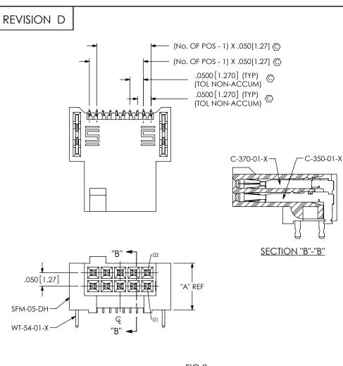
FIG 2 SFM-105-02-X-DH SHOWN (DIFFERENT AS SHOWN, OTHERWISE SAME AS FIG 1)
