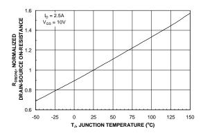
Figure 3. On-Resistance Variation withTemperature.
