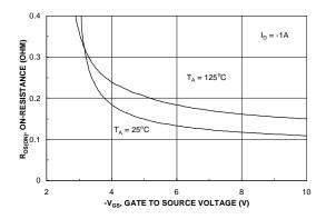
Figure 13. On-Resistance Variation withTemperature.
