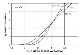
Figure 5. Transfer Characteristics.
