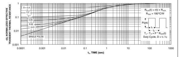
Figure 21. Transient Thermal Response Curve.
