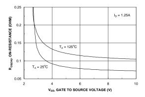
Figure 4. On-Resistance Variation with Gate-to-Source Voltage.
